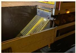
An agency operative working on his company supplied IPV suffered a trapping injury to his ankle due to the cone well cover collapsing and trapping his ankle against the structure of the vehicle.
